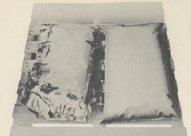
Kordite Heavy Duty Polyethylene bag (6 mil) and 4 ply paper bag containing Calcium Hypochlorite stored for 3 weeks. Paper bag was completely corroded, polyethylene bag showed no signs of corrosion.
